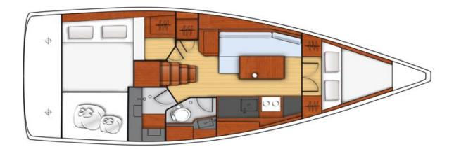
yanmar 30 HP shipyard: Beneteau engine launghed: 2017 fuel tank 130 lt. length over all: 10,45 m drinking water tank: 330 lt. length of the hull: 9,97 m berths: 4 + 2 width: cabins 3,72 m 2 draft: 1.45 m salon: Convertible head + shower 1 + 1
