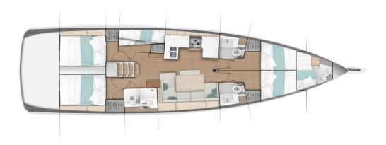
Shipyard: Jeanneau **Engine:** 80 HP Fuel tank: It. 240 Launched: 2023 Water Tank: It. 640 Length overall: 14.42 m Berths: 12 max Length of the hull: 14.00 m Cabins: 5 + 1 skipper Width 4.49 m Salon: convertible 2.24 m Draft Sail Area: ca. 109 m<sup>2</sup> Heads: 3 + 1 skipper
